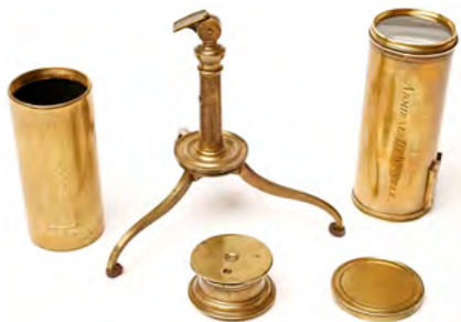
tripod legs fold up and all components store within the optical tube
