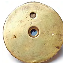
4-lens turret with solar filter
