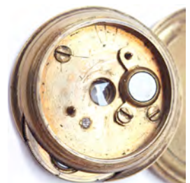
4-lens turret with solar filter
