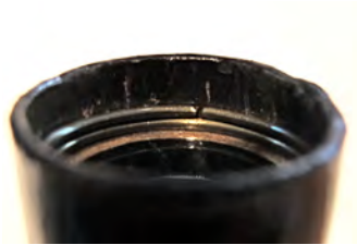
Masatomi: Eyepiece lenses held by 2 brass wire expansion rings
