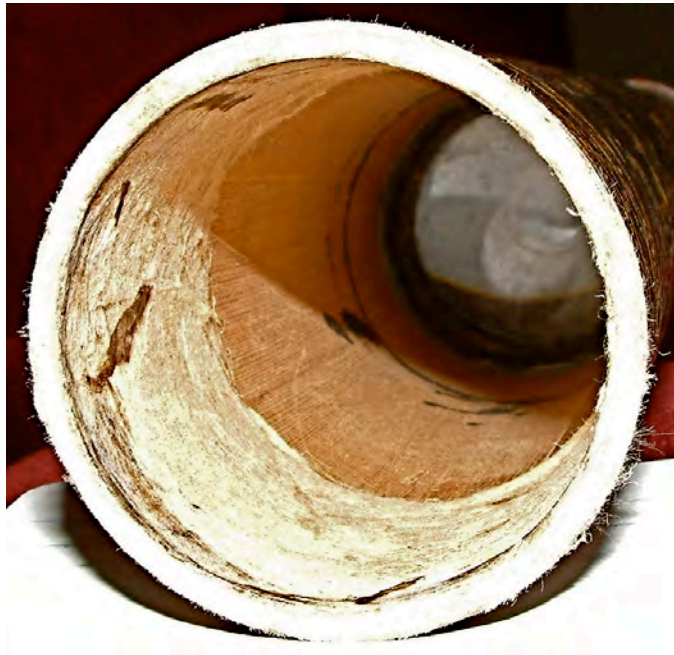
Non-stave construction of tubes
