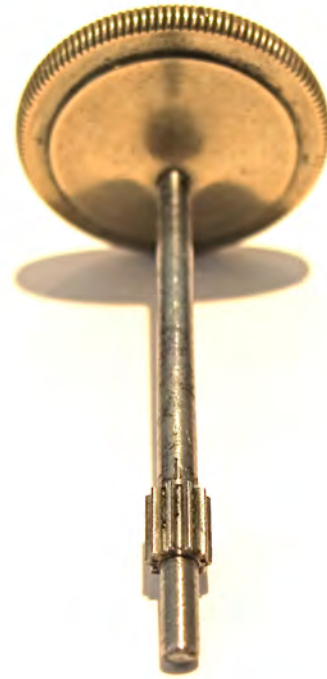
Right: Repaired pinion gear.
