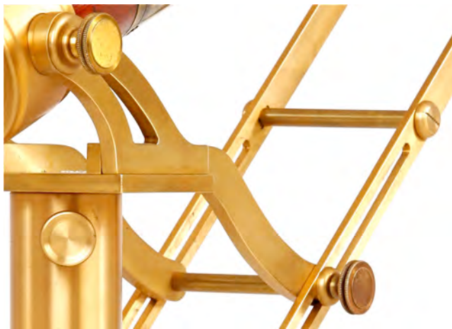
Altitude adjuster with tension bolt
