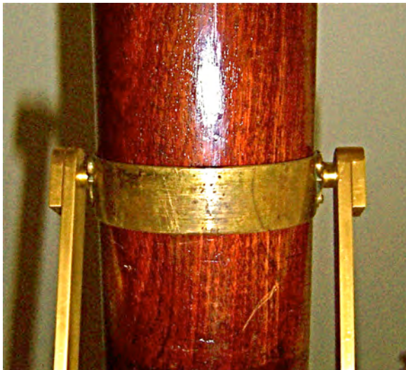
Original brass band with attachment knobs midway up second tube to which the flat brass struts were later attached.
