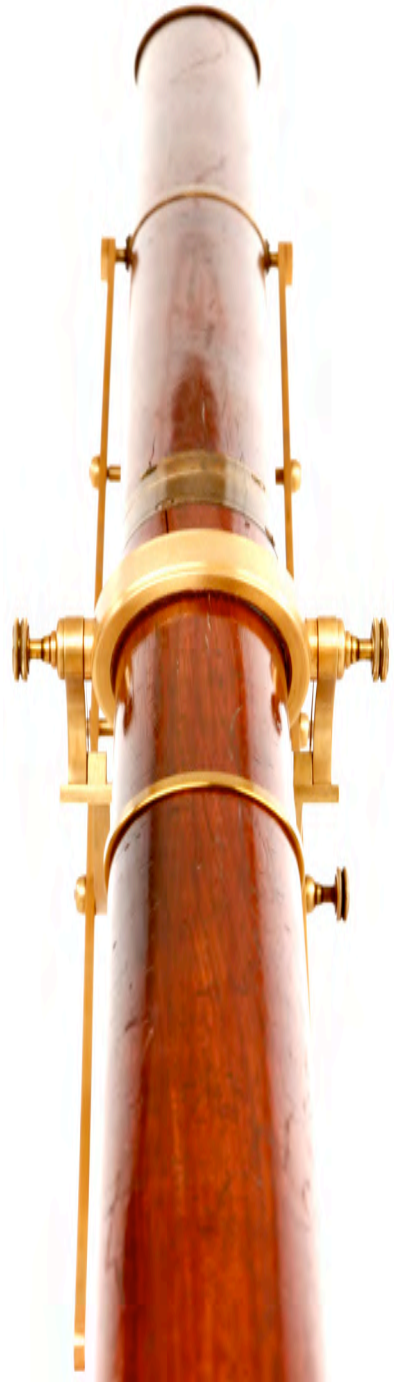
Up-the-tub view showing the pivot points (utilized 3 wire-knurling stubby Dollond bolts). this perspective does not show the taper.
