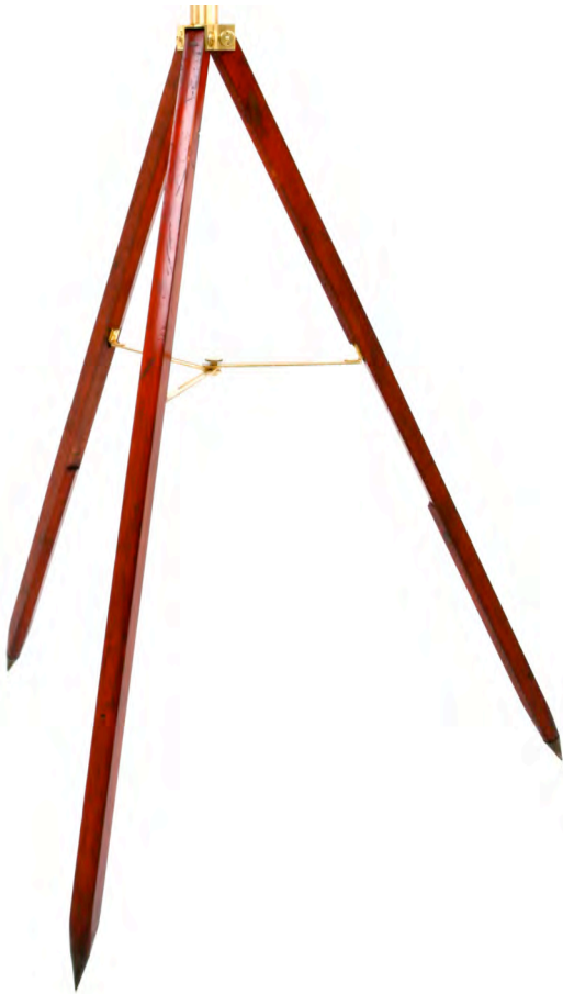
Adapted tripod with custom spider
