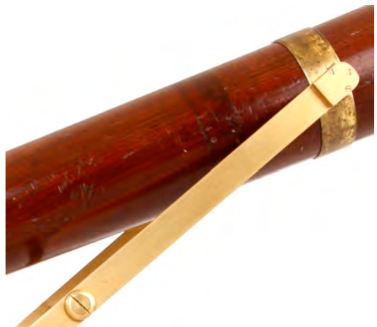
Pivot bracket and original collar midway up the second optical tube supports the upper section of the telescope
