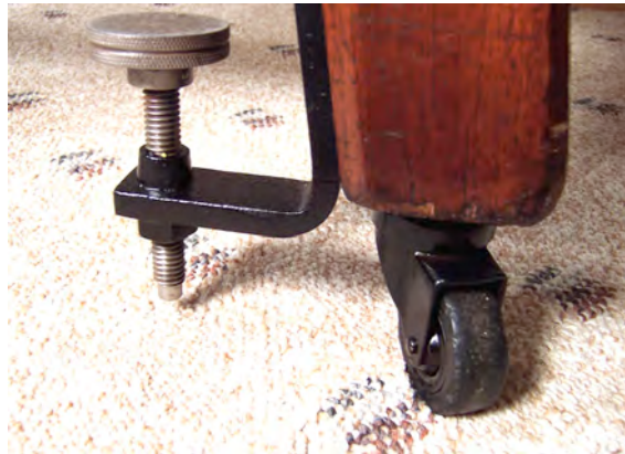
Straightened, cleaned and repainted with black satin enamel
