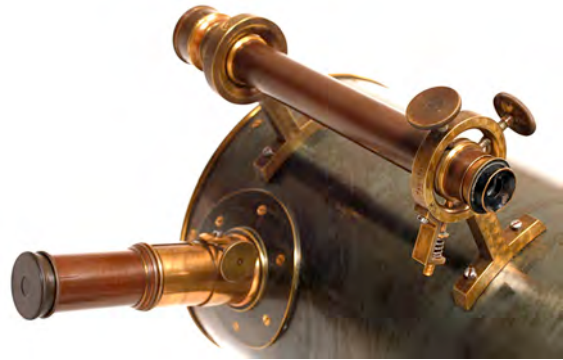
Replaced missing eyepiece in finder scope
