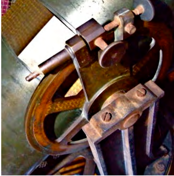
Declination adjuster and setting circle
