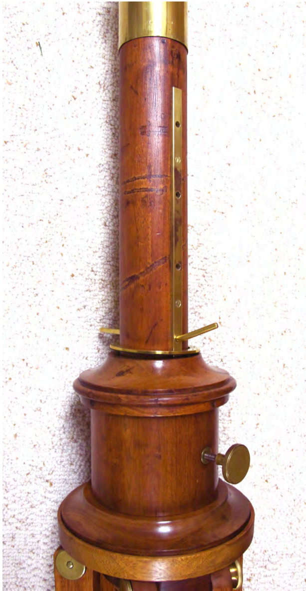
1/4-inch thick brass strip inlaid in old rack track with brass keeper pin and heavy brass disk for supporting the 90 lb. OTA; This arrangement provides the height adjustment for the 135-mm SECRETAN refracting telescope
