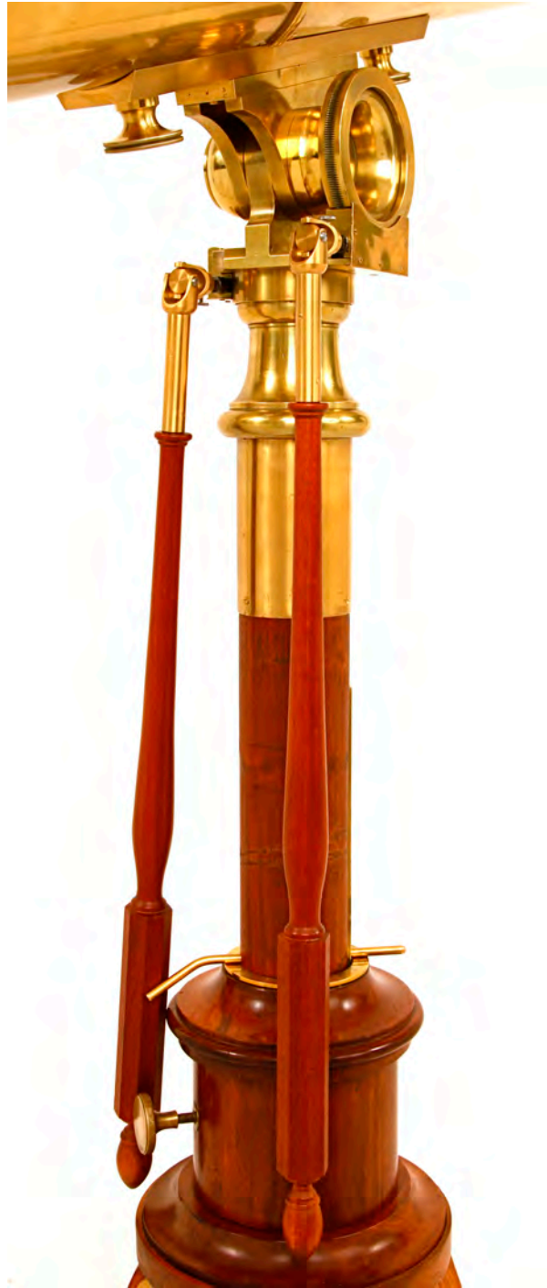
New custom replacement brass and mahogany slow motion control rods - after staining/finishing.
