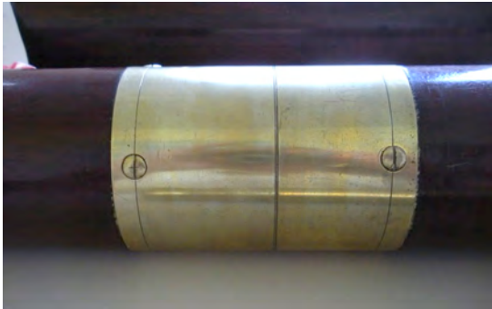
Brass coupler for upper/lower sections No mounting bolts on telescope
