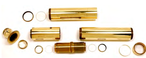
12-ft Dollond: 5-lens and 6-tube assembly (One tube is missing; a retrofit end-cap holds lens #1)
