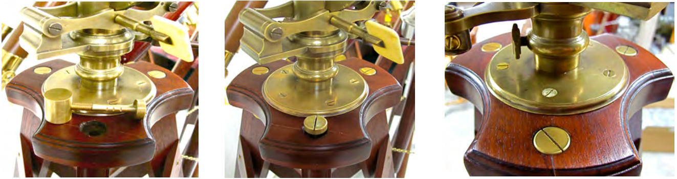
Three custom brass slotted cylinder-head tie-down bolts and three flush-mount cross-tie threaded keeper rods were fabricated. (left photo shows one of the units laying on the tripod plate, center partially tightened, right shows fully installed) Detail of base-plate attachment to tripod legs
