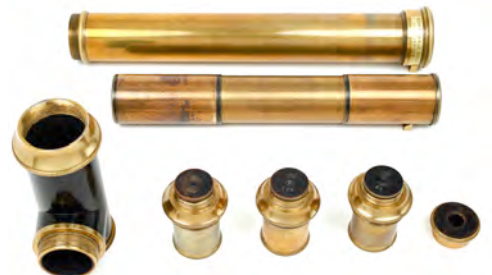
terrestrial eyepiece (top); star diag. & 3 celestial eyepieces
