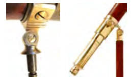
Eyepiece has orig. staff coupler and rack & pinion focus
