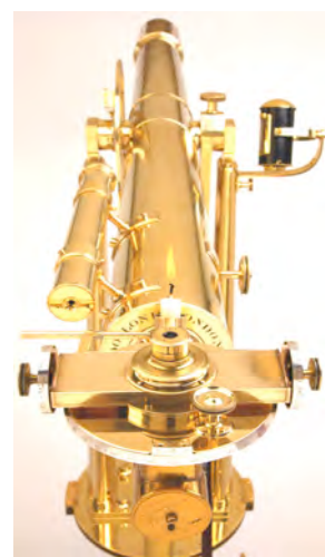
Candle-illuminated Troughton & Simms filar micrometer
