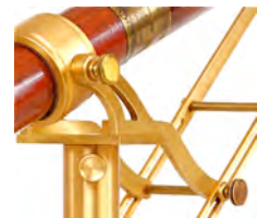
Viewing altitude angle set by tilting the tube to the desired angle and then tightening knurled compression thumbnut
