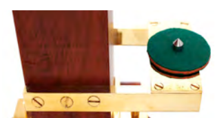
counter-weight resting platform with centering pin
