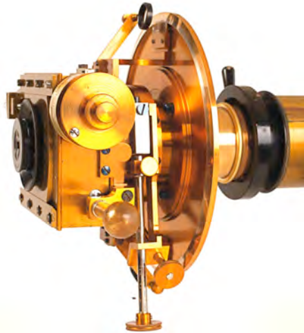
Heyde (Dresden) multi-wire filar micrometer
