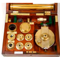
T&S 3-wire filar micrometer w/ candle illuminator 7-celestial and 1 terrestrial lenses w/adapters
