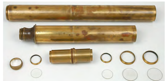
4 of the 5 eyepiece lenses are un-mounted and held in place by capture. Only the first lens is secured in a spun brass cell
