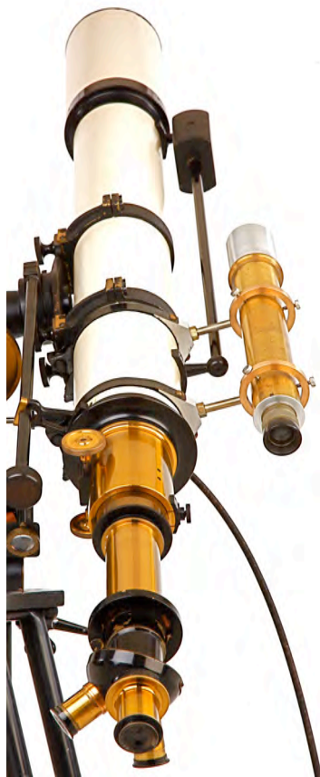
Heyde (Dresden) multi-wire filar micrometer
