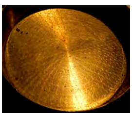
Brass objective lens caps with similar radial tooling marks on inside Unsigned: single scroll HRA30 Lerebours et Secretan Opposing double scroll
