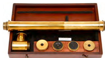
Dollond 5-lens set with star diagonal with pancratic terrestrial lens
