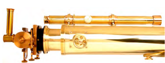
Unsigned Grubb multi-wire filar micrometer mounted in its case with several accessories as well as three celestial telescope eyepieces: F.L.= 2.7" Kellner and F.L.= 1.5" & 0.65" Huyghenian eyepieces
