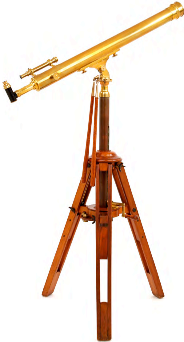
slow motion control rods and worm gear driven elevator for raising and lowering telescope
