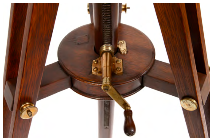
worm gear lifts the center shaft to raise and lower telescope
