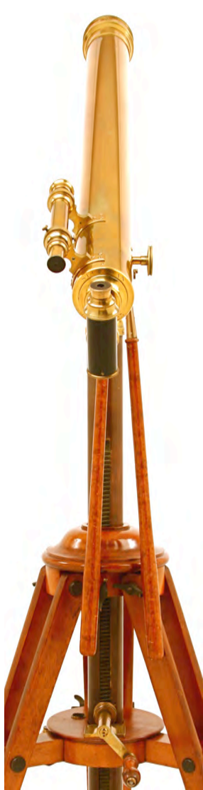
slow motion control rods and worm gear driven elevator for raising and lowering telescope
