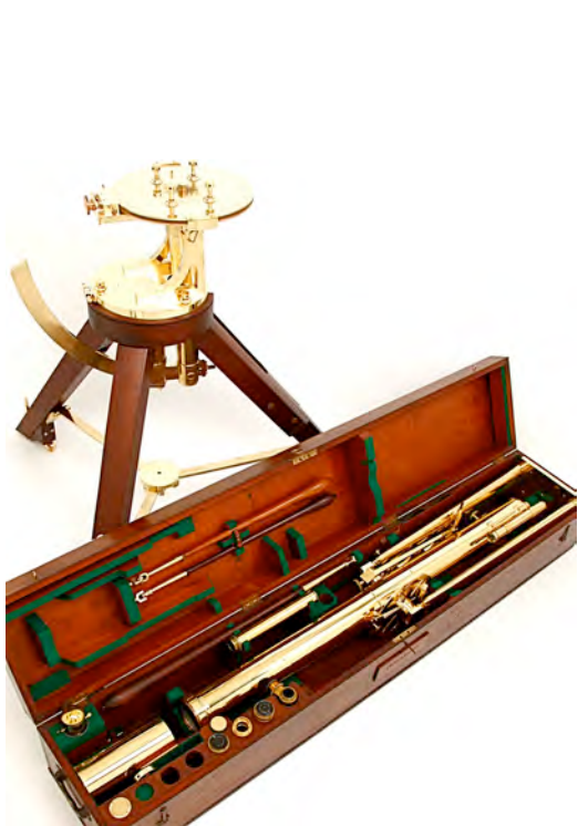
Massive mahogany case (6'x1'x1') stores telescope down to trunnion bottom of plate, lens set, spectroscope, oil lamp, and adjusters
