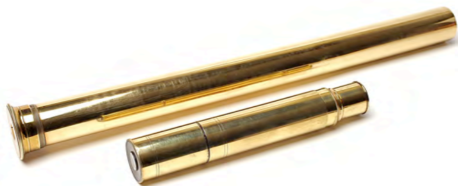
eyepiece assembled but not inserted into eyepiece tube
