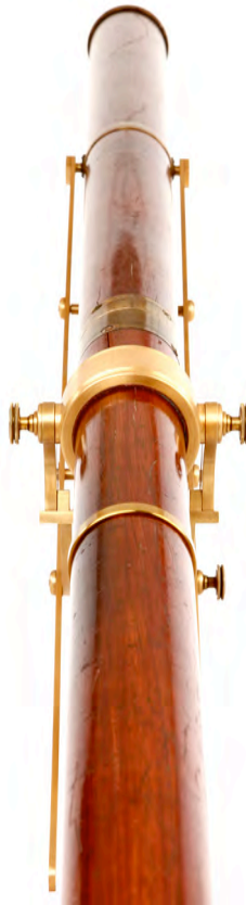
Viewing altitude angle set by tilting the tube to the desired angle and then tightening knurled compression thumbnut
