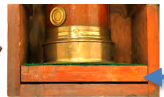
Leather washer separates end boards for shock protection
