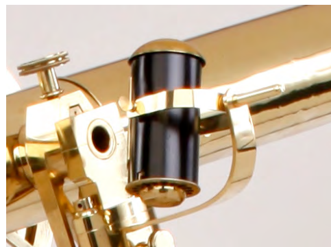
Oil lamp is gimballed-mounted at the pivot on the transit mount and mid-point on the OTA
