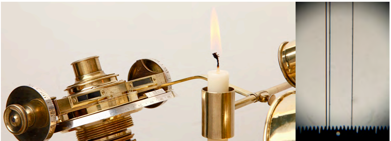
After: Note glass windows on front edge of the T&S micrometer for the candle illumination to enter Single wire (left), double (right)
