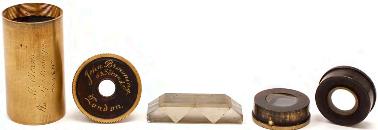
John Browning/McCleans Star Spectroscope (Before and after - no restoration or adaptation required!)
