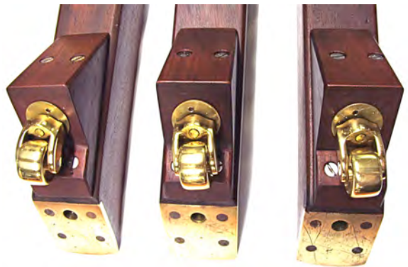
New solid brass casters mounted on heavy mahogany mount blocks required for the 350 lb. load (> 100lb./caster)
