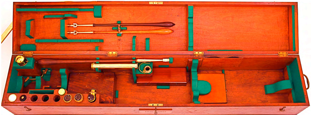
Storage case open without telescope: accessories cases left to right across the bottom of the case include John Browning McClean's Star Spectroscope, Troughton & Simms filar micrometer, Dollond lens set, and John Browning split-lens micrometer
