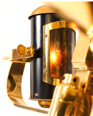
Restored Dollond oil lamp is lit. It burns brightly behind its old original mica window with its new rope wick
