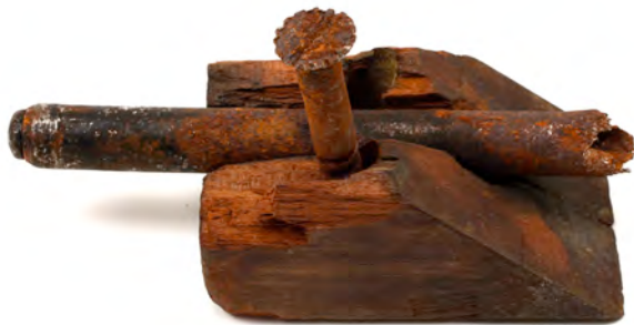
Pieces of original caster block, receiving sleeve for caster pin and one wood screw for holding the caster block
