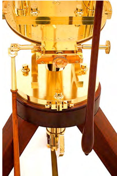
Mahogany tripod base supporting transit trunnions mounted on a large tiltable universal equatorial plate
