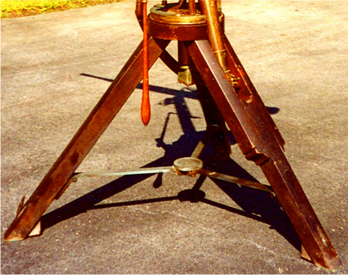
Note the bent, broken, and missing leveling bolts and missing brass casters and floor-leveling bolt adjuster
