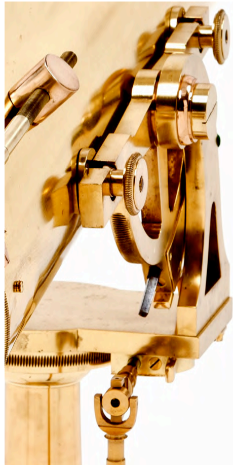
Rear view of the stacked adjuster connections
