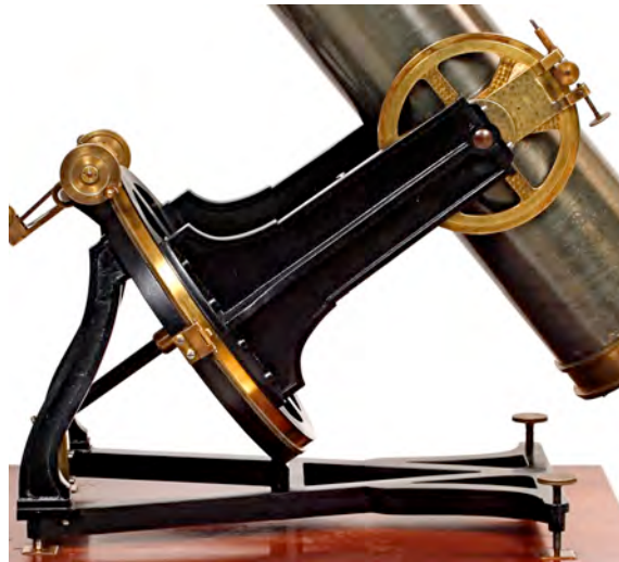
TRE17: SECRETAN Coarse declination by manually tilting tube; fine adjustment by linear screw.
