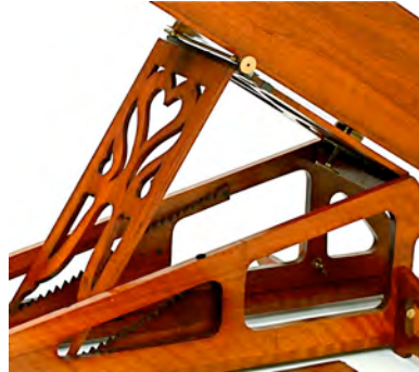
▲ Coarse 2°/notch <- Altitude adjusters -> Fine Thumb Screw ▲
