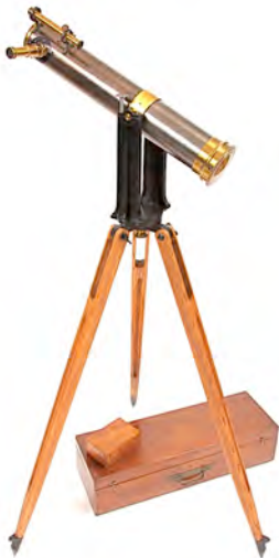
FRE1: SECRETAN Altitude and azimuth adjustment by manually tilting and turning the main tube, respectively.
