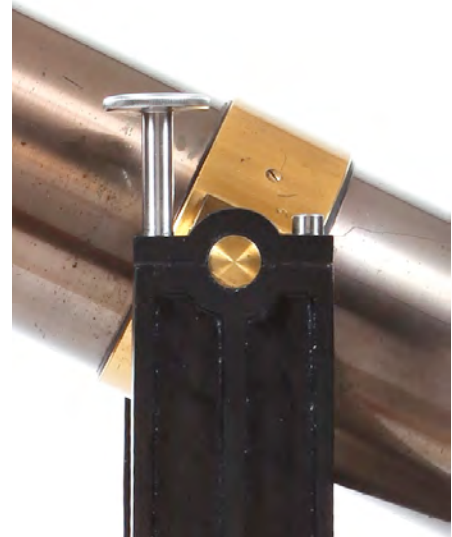
FRE1: SECRETAN Altitude and azimuth adjustment by manually tilting and turning the main tube, respectively.
