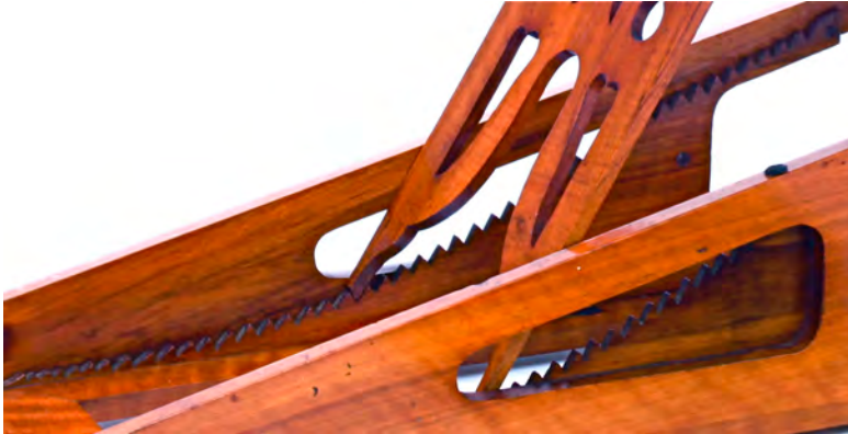
TRE16 Altitude: Coarse Adj. 2°/ notch by lifting tube
