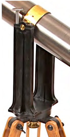
FRE1: SECRETAN Altitude and azimuth adjustment by manually tilting and turning the main tube, respectively.
