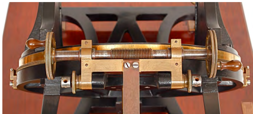
TRE17 Right Ascension: Manual fine crank adjustment
