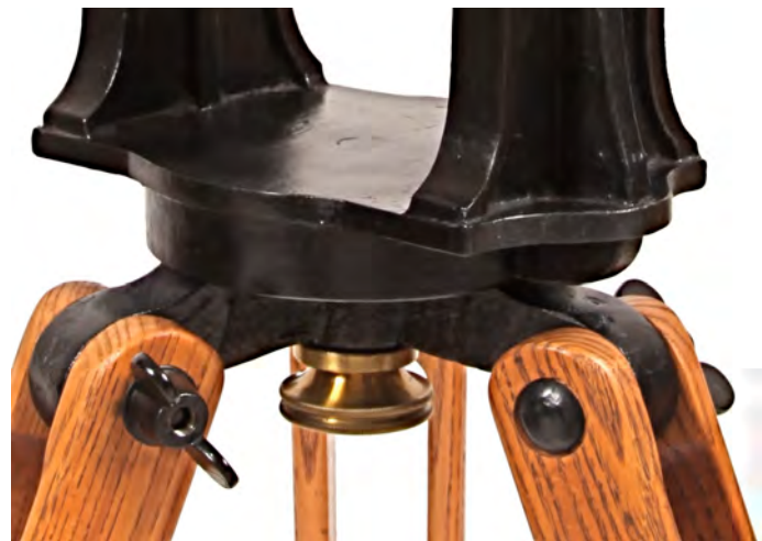
Azimuth: Manually turn transit-type mount
