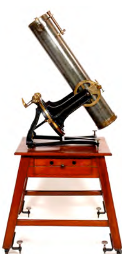
TRE17: SECRETAN Coarse declination by manually tilting tube; fine adjustment by linear screw.
