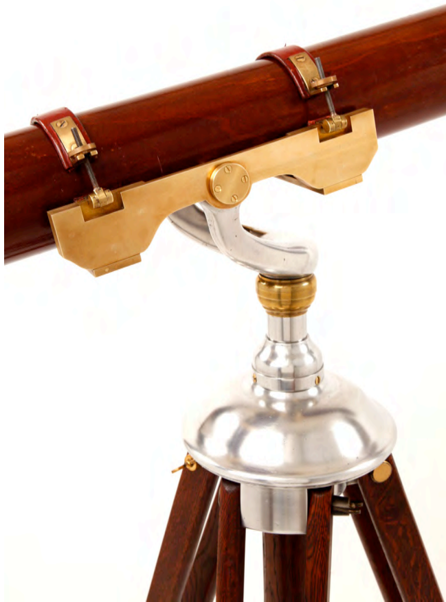
As restored: Used the original leather-clad Secretan compression bands with knurl brass nuts and a custom designed and fabricated brass "trough" mount to adapt the older telescope to a more recent tripod with an aluminum altazimuth pivot mount.
