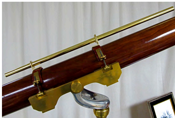
Custom designed and fabricated mechanical finder, which is a collapsible and adjustable brass sighting tube with cross hairs.
