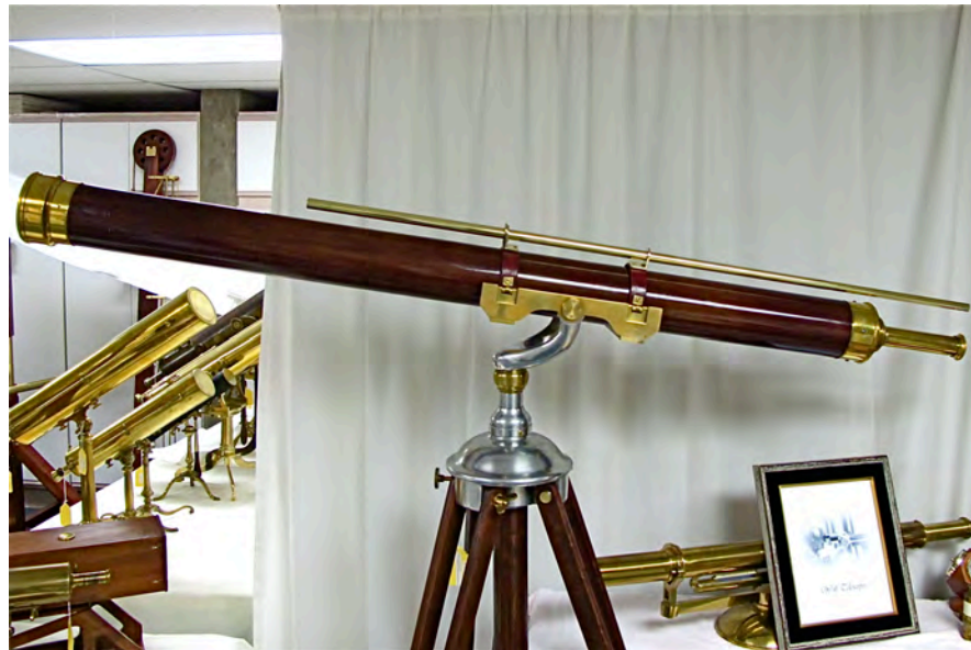
Beautiful "marriage" of Lerebours et Secretan telescope, c. 1865 and Secretan tripod, c. 1915 utilizing a custom tough mount adaptation with the addition of a novel finder sighting tube.
