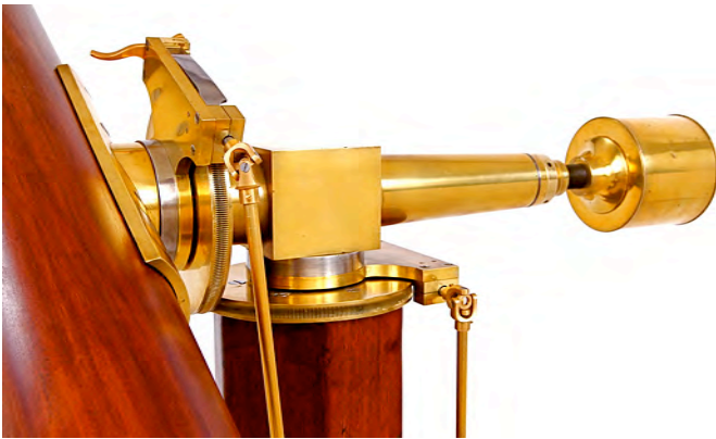
After: Beautiful original wood revealed (walnut tube and mahogany tripod) and new restored brass control rods. New control rods designed from remaining original swivel (below) and photos of same period Merz - fabricated from mahogany and brass.
