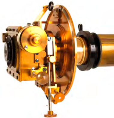
Threaded Zeiss tube sized and soldered to Heyde micrometer mounting plate
